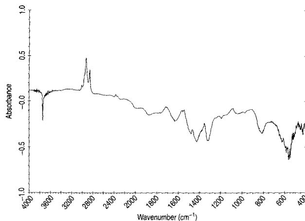
FIG. 6. The Fourier transform infrared spectra of rice hull ash (RHA) incubated for 15 min with 100 mL of 0.05M oleic acid and 0.05M isopropanol in hexane and subsequently washed with 100 mL hexane. The spectrum of RHA has been subtracted.
