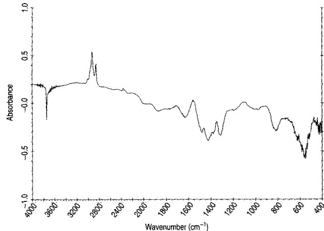
FIG. 5. The Fourier transform infrared spectra of rice hull ash (RHA) incubated for 15 min with 100 mL of 0.05M oleic acid in hexane and subsequently washed with 100 mL of 0.05M isopropanol in hexane. The spectrum of RHA has been subtracted.
